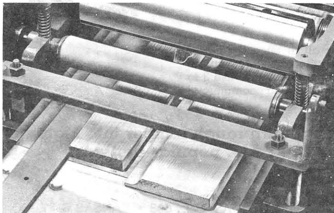
FACE MOLDING —This board is emerging from the new Belsaw, sawed to width, planed to the desired thickness and molded for baseboard use, all with power feed.
